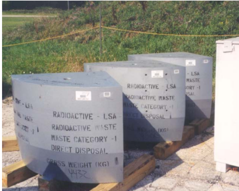
Fig 9 – Photo of sections from the upper magnetic pole of the ANL Bldg 211 Cyclotron. Each section weighed roughly 9,750 pounds
