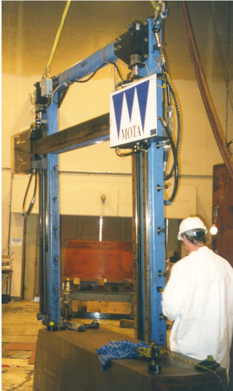
Figure 1 – MOTA Corporation's Reciprocating Machine Tool in field use at Argonne National Laboratory Bldg. 211 Cyclotron D&D Project.
