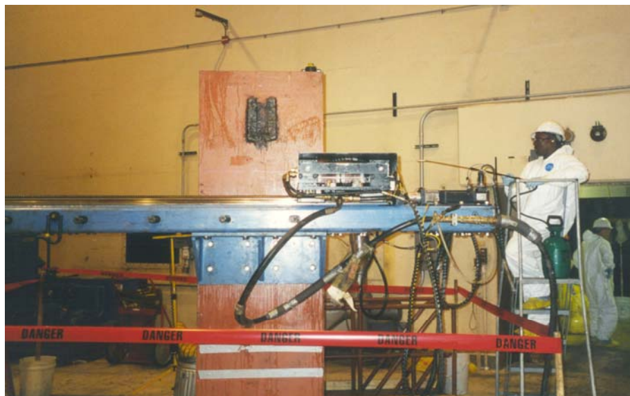
Fig 10 – Photo of the MOTA Reciprocating Machine Tool mounted horizontally on the North side post of the Bldg. 211 Cyclotron
